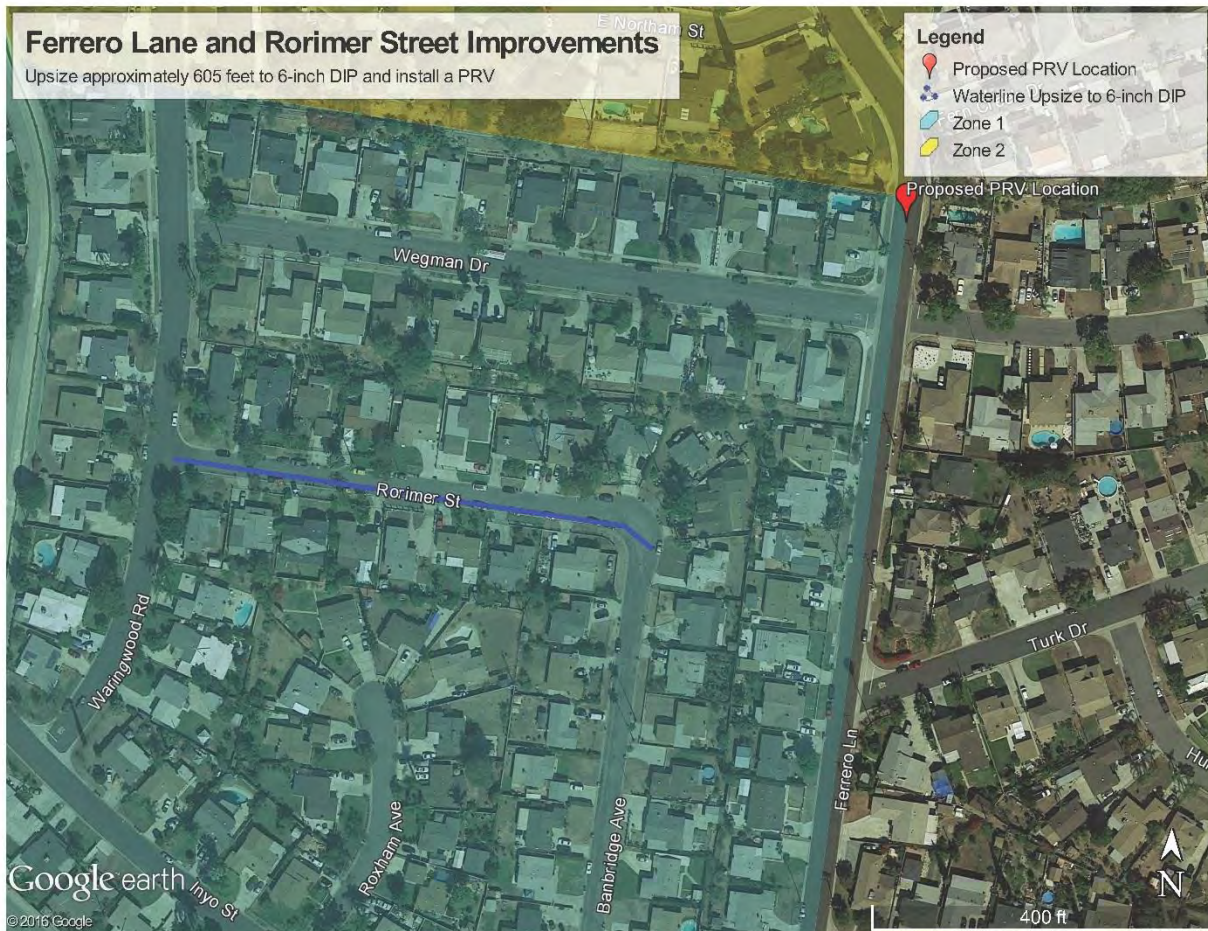
Figure 9-10 – Ferrero Lane and Rorimer Street Improvements (CIP#2)
