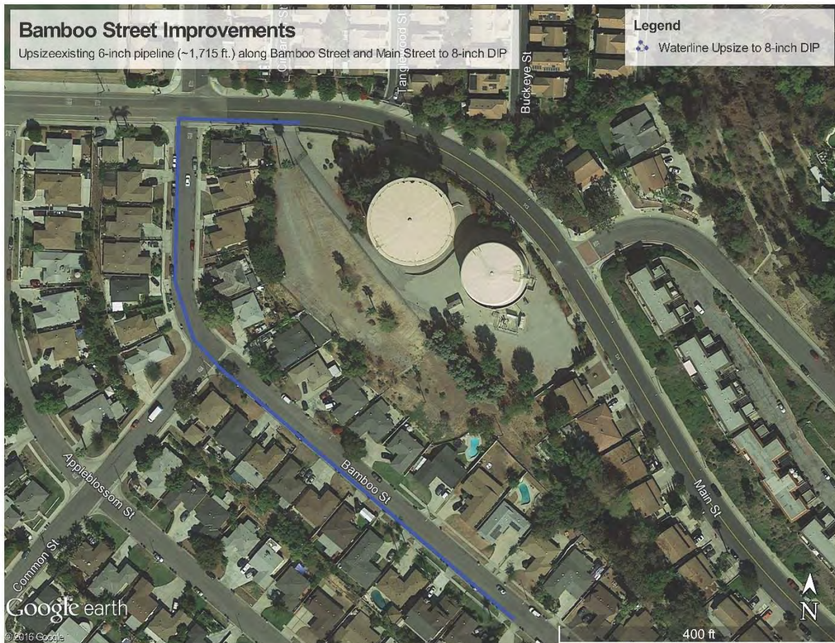
Figure 9-14 – Bamboo Street Improvements (CIP#6)
