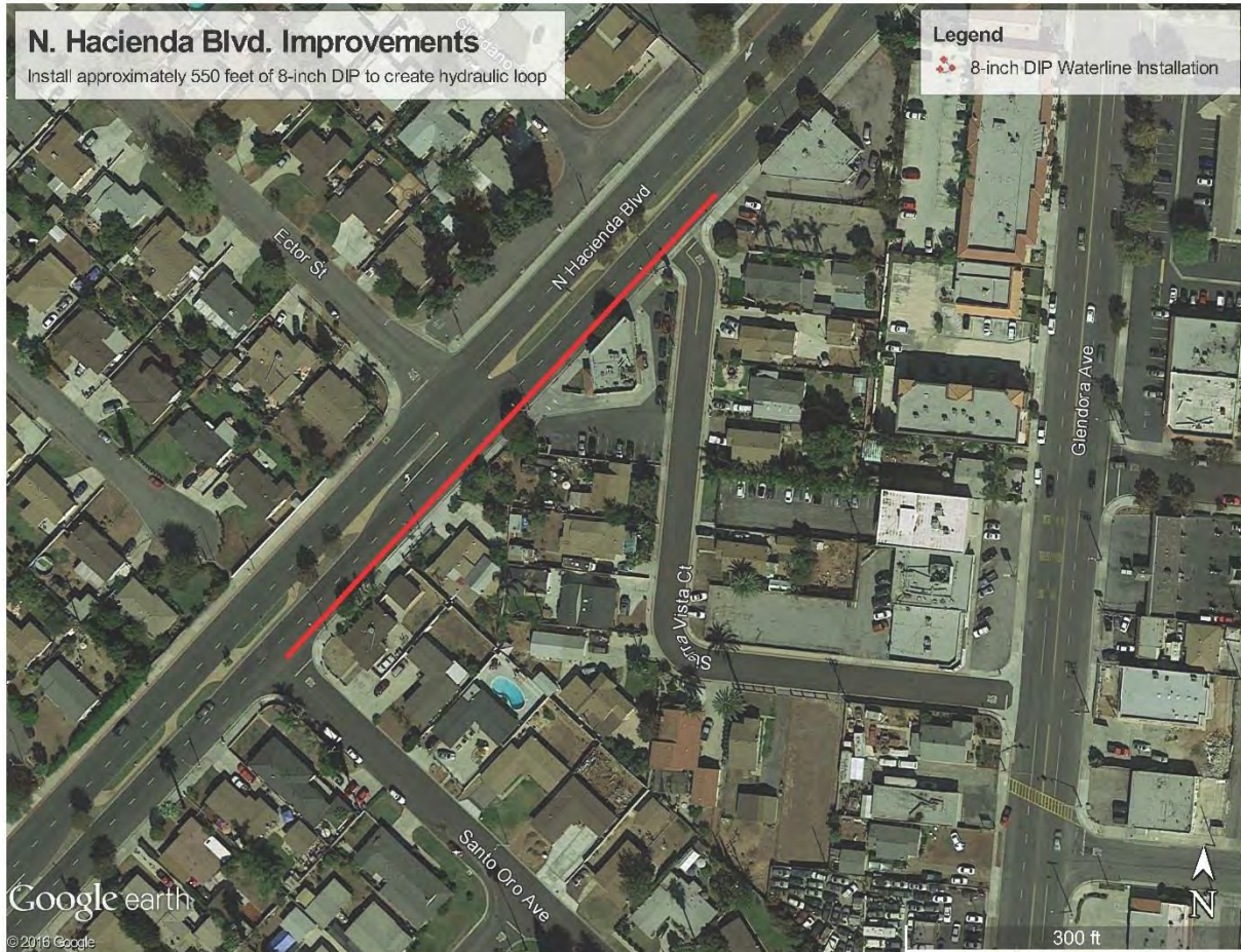
Figure 9-13 –N Hacienda Blvd, north of Temple Ave Improvement (CIP#5)
